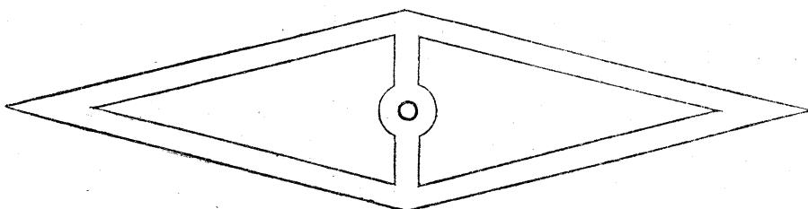
In ascertaining the directive force, the balance of torsion of M. COULOMB was employed. This instrument, as is well known, consists of a fine wire attached to an index moveable round a circle, divided into degrees. To the other end of the wire is fixed a cradle, to receive the needle which is the sub-
